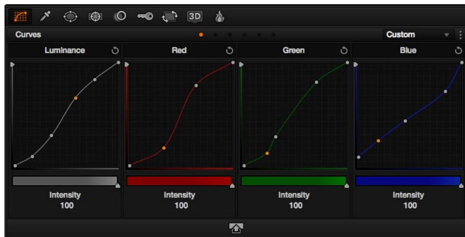
Turning off curve ganging lets you independently adjust each curve
