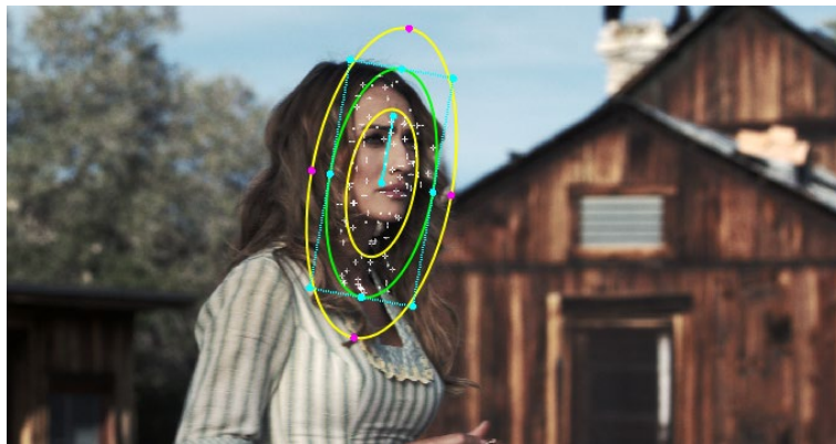
Object tracking in progress. Tracking points are automatically placed over trackable features of the image
