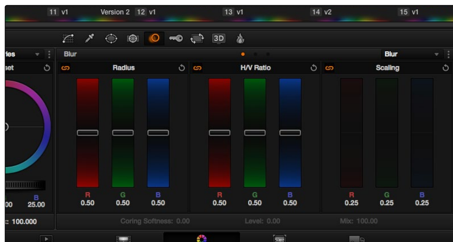
Blur Radius controls are ganged by default, but can be unganged
