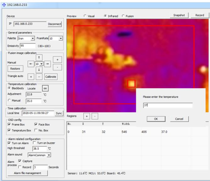
**Step 7** Check whether the infrared image is aligned with the visible light image. If it is not correct, you can adjust the fusion image calibration appropriately. If the alignment is abnormal, the temperature measurement will be inaccurate.
