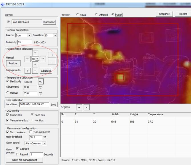
**Step 8** Configure alarm information, select infrared video, add an alarm area (draw a frame in the infrared video image, you can select the required frame according to the size of the alarm area required), start the alarm service, and fill in the alarm threshold temperature.
