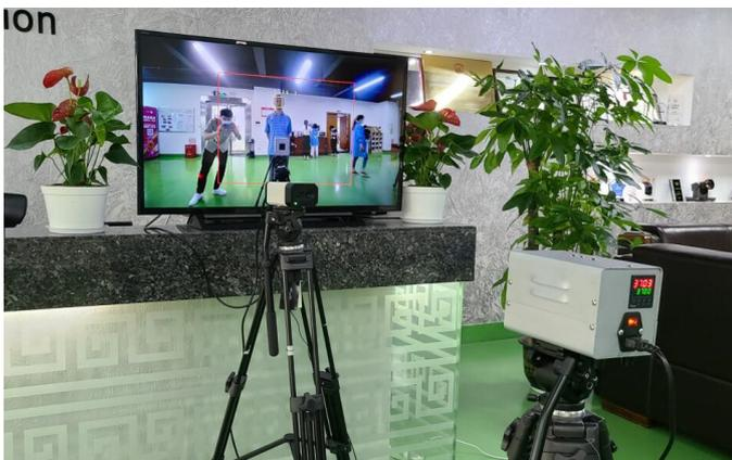
**Step 3** Set the heating temperature of the blackbody to 37°.
