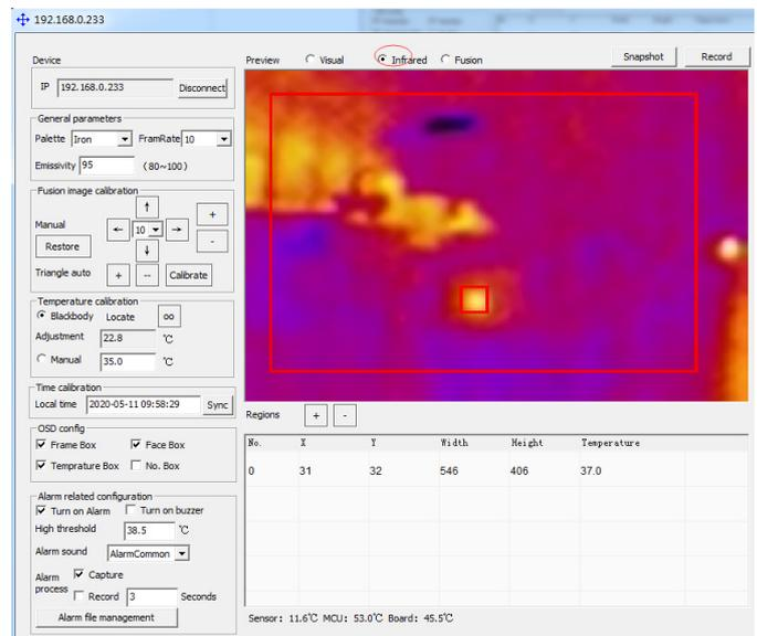
**Step 6** Configure the blackbody parameters in the camera, enter the emissivity 95, select the blackbody temperature calibration, and click the OO button to
