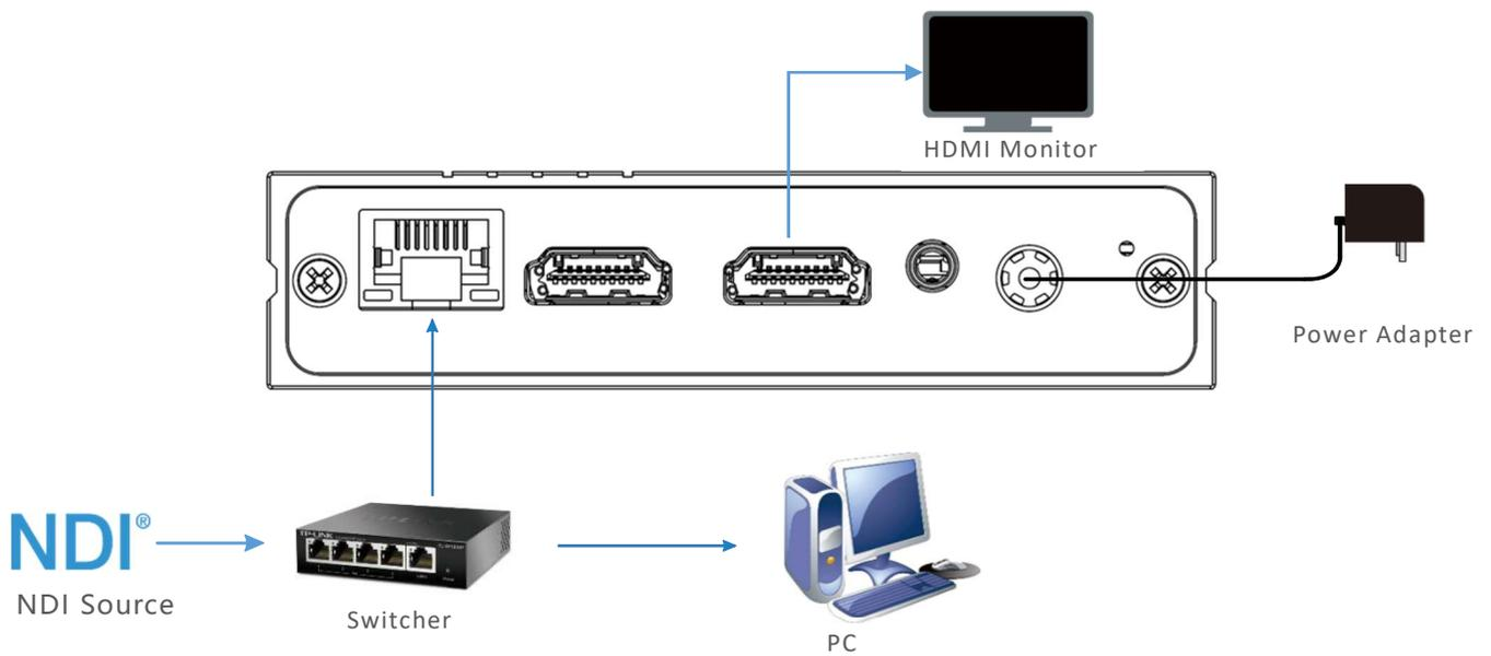
Decoding mode application system connection diagram
