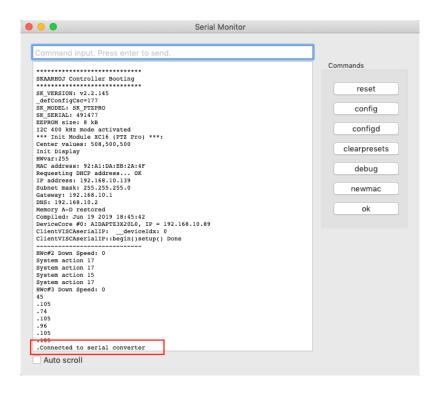
In order to verify connection to the camera the Serial Monitor must state the below commands
